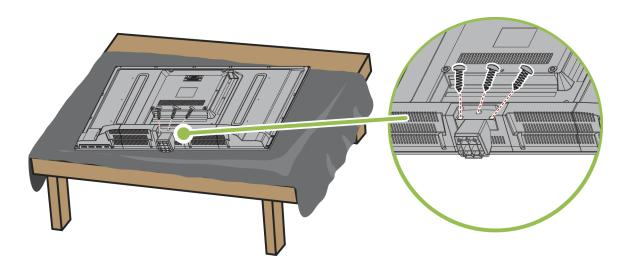
3 Attach the TV stand to the stand column with four of the provided M4 (12 mm) screws.
